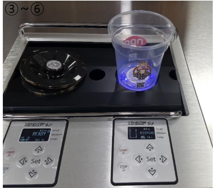
* Insert a cup to check LED, Solenoid valve functions correctly, and check all buttons work fine.
